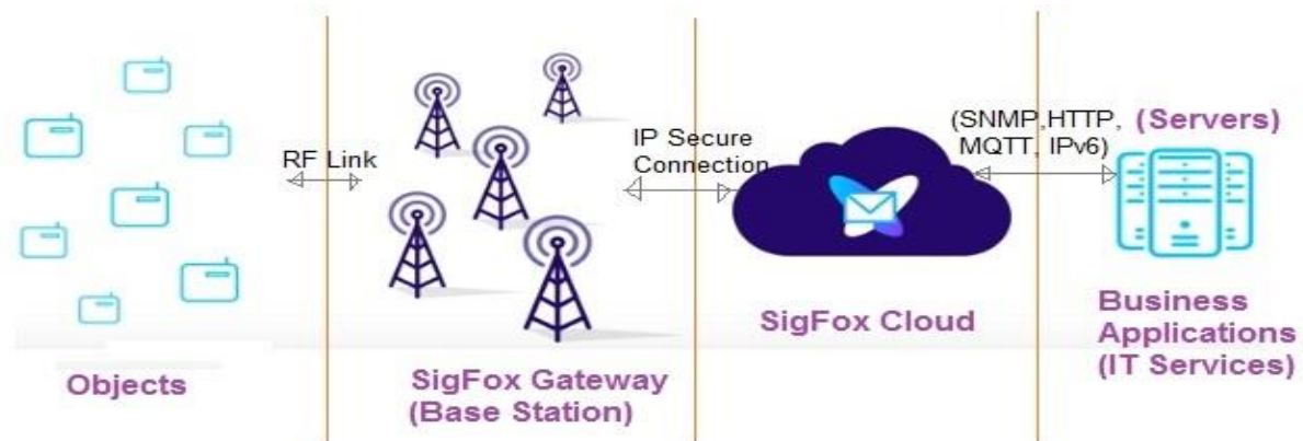
Figure 11: SigFox network architecture
